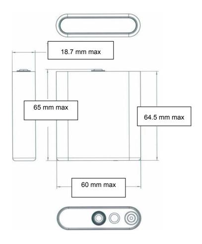
For information only since the MP 176065 cell is not marketed as is, but only when fitted with its individual protection circuit, thermal fuse and external sleeving.
