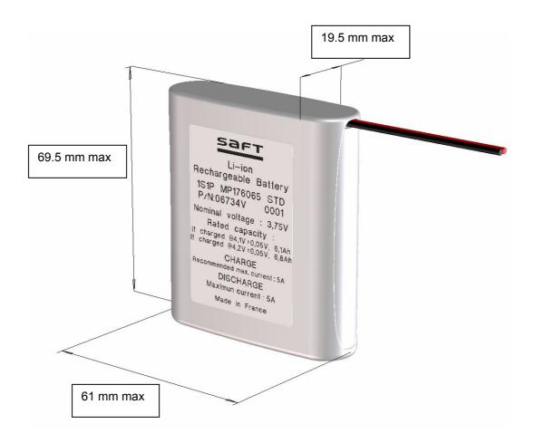
**NOTA:** The thickness 19.5 mm max. corresponds to uncycled batteries. 0.9 mm to be added for batteries cycled 500 times.
